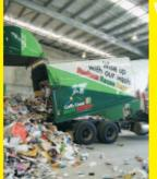
A. Receival area and incline conveyor Trucks drop the recyclable material onto the receival floor.
